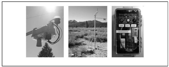
Figure 6.1: A Snowcloud Sensor Node (L,C) and Harvester Device (R).
